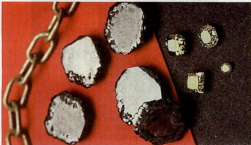
A CUT ABOVE Apollo uses chemical vapor deposition to grow plates of very pure diamond (left) that can be cut and polished into beautiful gems (right).
